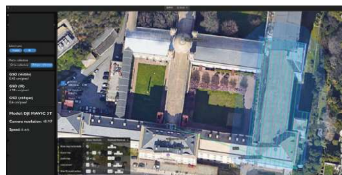
Figure 4. Screenshot from DJI FlightHub 2 showing the flight-plan for one of the roof coverings of the Albergo dei Poveri complex (Genoa).
