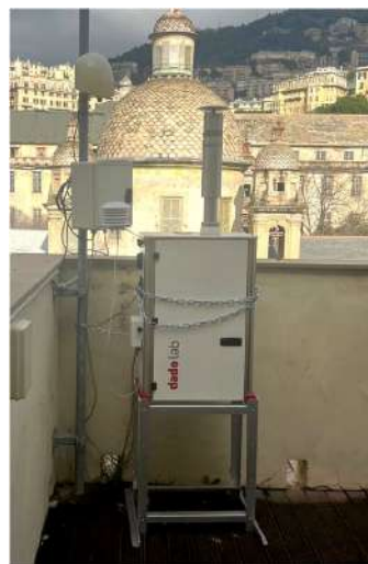
Figure 2. Environmental monitoring instrument (IoT air quality monitoring) installed inside the experimental case study site, the Albergo dei Poveri complex (Genoa).
