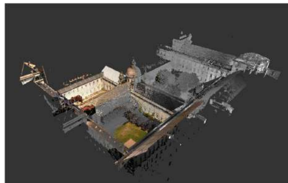
Figure 6. Visualization of the point cloud processed through tLS within Autodesk ReCap Pro 2025 software.
